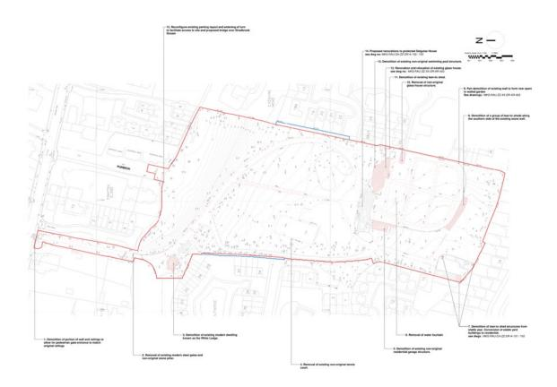
Figure 13 – Extent of Demolition (Existing Site Plan)
